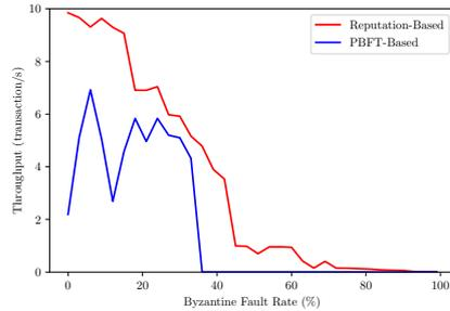
**Figure 10:** Throughput comparison between delegated consensus-based blockchain and PBFT-based blockchain as the Byzantine fault rate increases.
