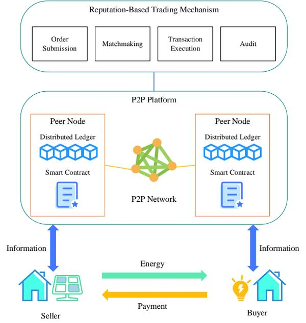
**Figure 5:** Architecture of P2P energy trading system based on blockchain and reputation.
