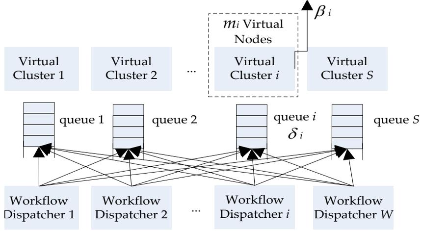
Figure 2. A queuing model of the VM resource allocation system for a virtualized cloud platform. Multiple workflow dispatchers are employed to distribute tasks to various queues. Each virtual cluster uses a dedicated queue to receive the incoming tasks from various workflows. The number of VMs (or virtual nodes) in each virtual cluster is denoted by  $m_i$ . The service rate is denoted by  $\delta_i$  for queue  $i$ .
