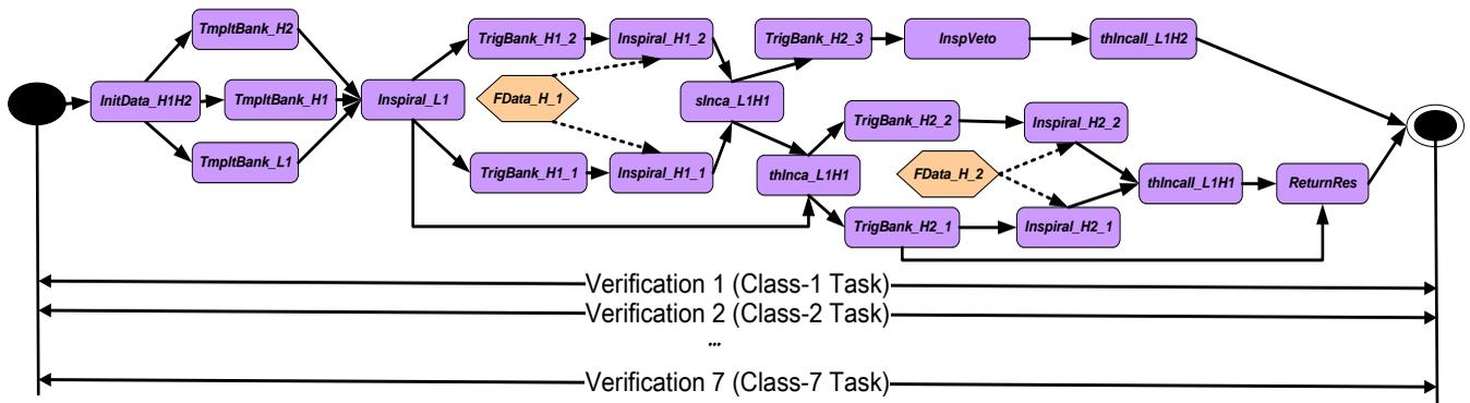
Figure 6. An example of resource allocation in many-task workflow for the LIGO workload, where the tasks are the 7 classes of verification programs running in parallel through the whole workflow.
