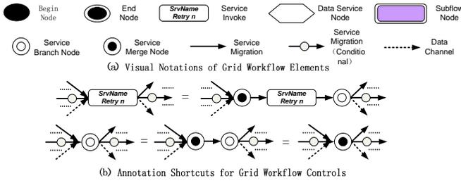
Fig. 1. Visualization of grid workflow elements
