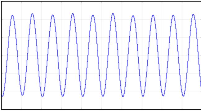
Fig. 10. Current waveform of a four voltage-level MMC
