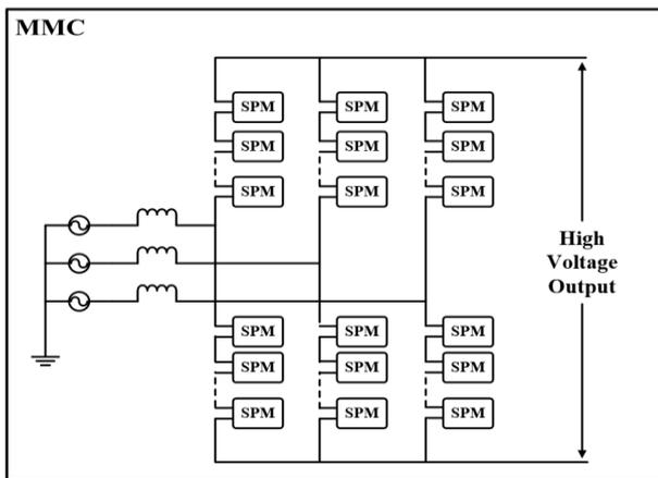
Fig. 7. Topology of MMC made up of SPMs
