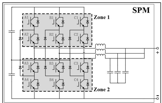
Fig. 8. Topology of sub module of MMC
