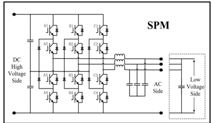
Fig. 1. Structure of SPM
