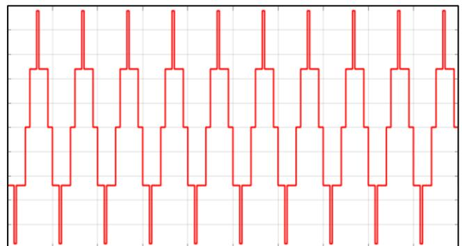
Fig. 9. Voltage waveform of a four voltage-level MMC
