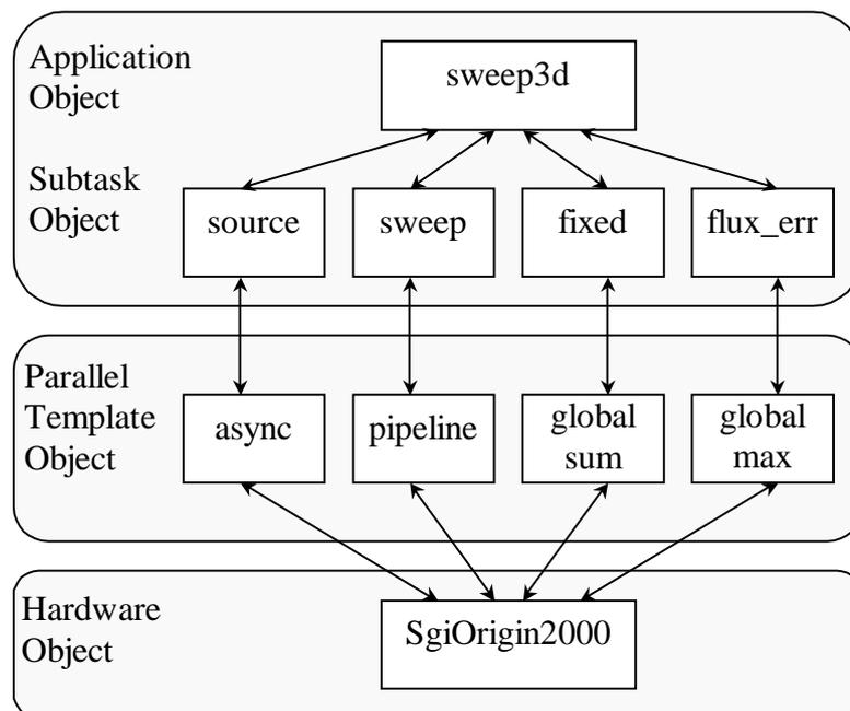
**Figure 4.2 Sweep3D Object Hierarchy (HLFD Diagram)**
