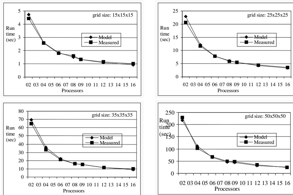
**Figure 4.7 PACE Model Validation on an SGI Origin2000**
