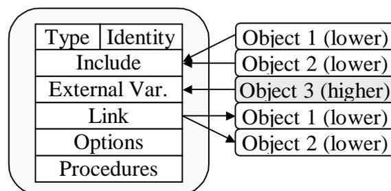
**Figure 2.2 Software Object Structure**
