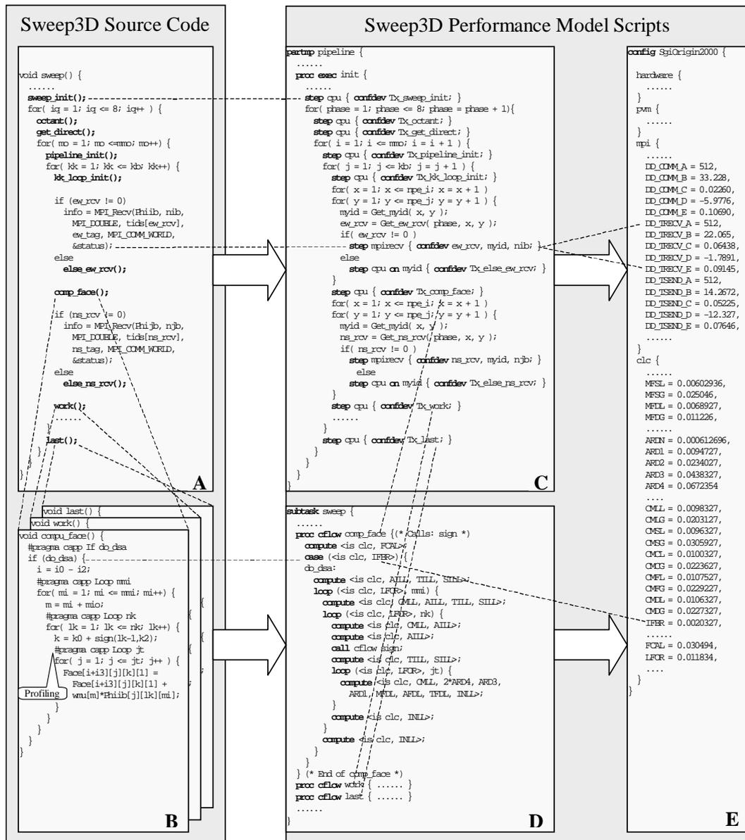
Figure 4.6 Mapping between Sweep3D Model Objects and C Source Code
